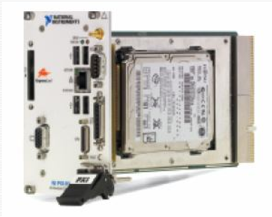
RT embedded NI PXI Controller (National Instruments)
