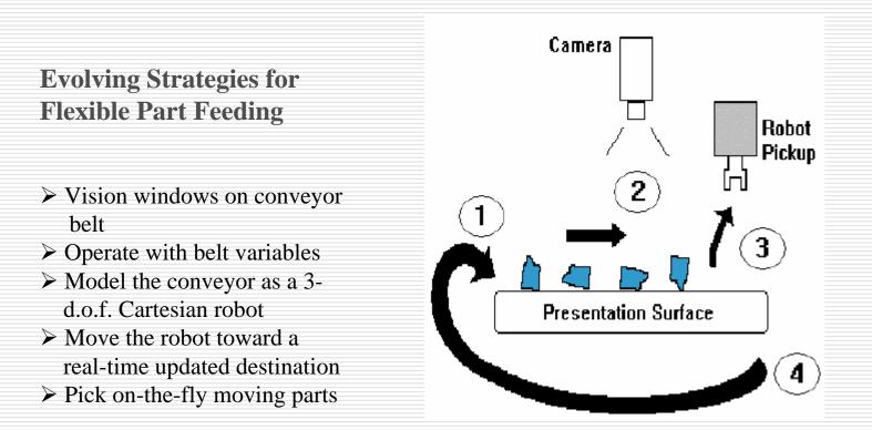
Basic flexible feeding concept: 1 – supply parts; 1 – locate desired parts; 3 – pick qualified parts; 4 – recycle parts that are not picked.
