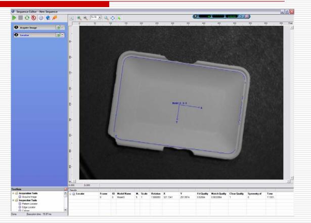
Recognizing interior shape of interest with *incomplete outer part contour* and *random position and orientation of entire object*
